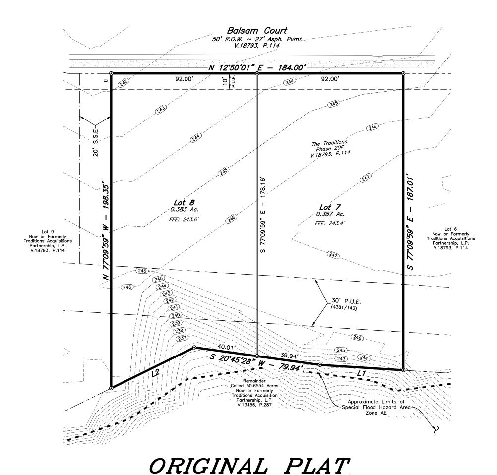
LINE TABLE LINE | BEARING | DISTANCE L1 S 16°28'55" W 52.55' L2 S 13'18'22" E 58.34'
